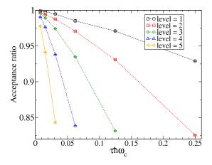
Acceptance ratio for a single particle, rectangular torus,  $N_{\phi} = 2$ flux quanta,  $\beta \hbar \omega_c = 2$ , and  $8 \le M \le 256$ .
